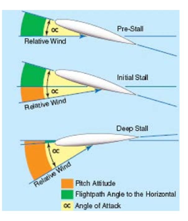
Dynamic stall process can be explained by a number of a stages.
